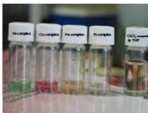
Figure 3. Perfect dispersion of nanoparticles in organic or aqueous solvents.
